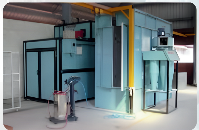
Batch type Powder Coating Plant
